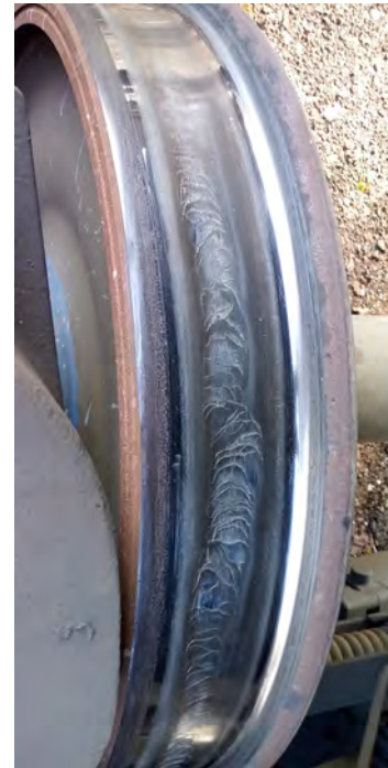
Figure 10: Example of wheelset damage on train 6A11 (photos courtesy of DB Cargo).
