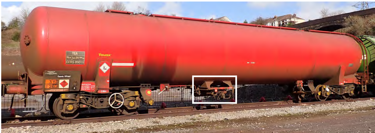
Figure 5: Wagon GERS89016 and its brake group (auxiliary reservoir hidden by brake group).
