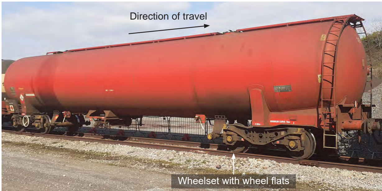
Figure 9: Wagon GERS89016 at Bristol East depot after the accident (photo courtesy of DB Cargo).
