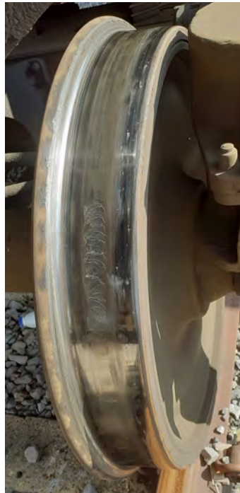
Figure 10: Example of wheelset damage on train 6A11 (photos courtesy of DB Cargo).
