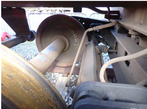
Figure 10: Example of wheelset damage on train 6A11 (photos courtesy of DB Cargo).
