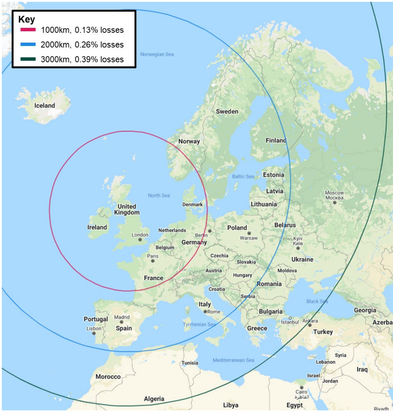
Figure 1 Map for determining which default factor to apply when calculating losses during pipeline transport. If the site of injection is within the circle, the specified losses factor for that circle shown in the key above may be applied. An interactive version of this map is available here (Source: mapdevelopers.com , Map Data: ©2021 Google, INEGI).
