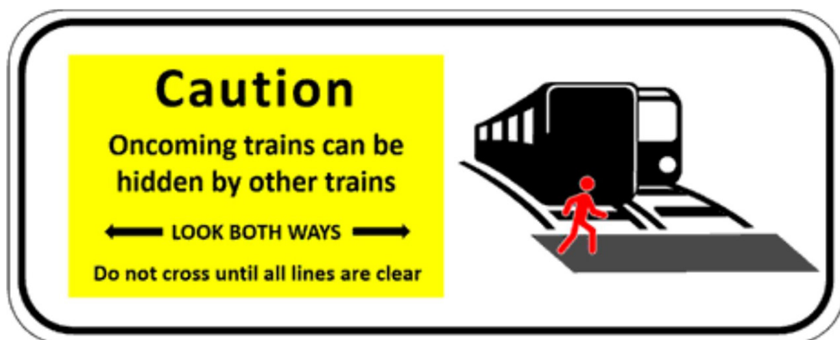
Figure 10: Design of sign to diagram 157 in the Private Crossings (Signs and Barriers) regulations 2023 (courtesy of HMSO).
