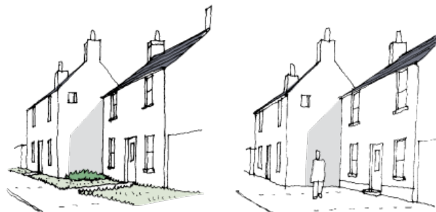
(Left) Indeterminate grassed or planted area in front visually detaches building from street to detriment of townscape (Right) A publicly accessible paved area forming part of the general street space
