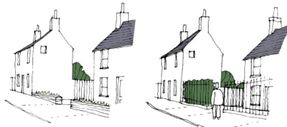
(Left) Indeterminate grassed or planted area in front visually detaches building from street to detriment of townscape (Right) A publicly accessible paved area forming part of the general street space
