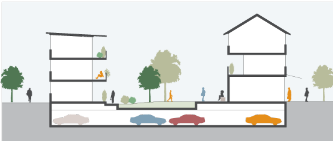
Underground parking with communal space above
