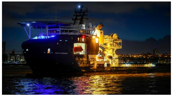
The 6,000-tonne, 98-metre-long offshore patrol vessel can handle a range of activities, including operating remote and autonomous off-board systems for underwater surveillance and seabed warfare. The Topaz Tangaroa is the first of two Multi-Role Ocean Surveillance (MROS) ships that will be operated by the Royal Fleet Auxiliary (RFA).
