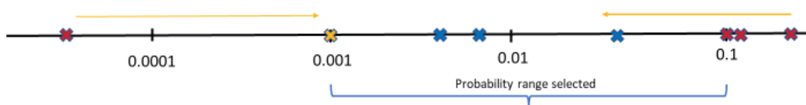
Figure 1 – Spread of active well seep leak data with selected range
