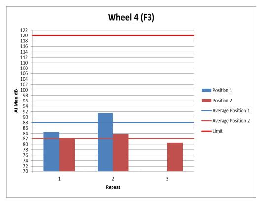
Figure 65: Individual Noise Levels for Wheel 4 (F3)
