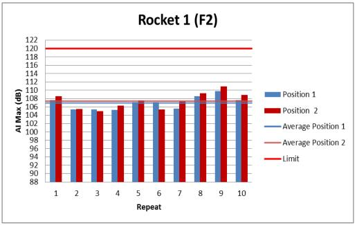
Figure 1: Individual noise levels for Rocket 1 (F2)
