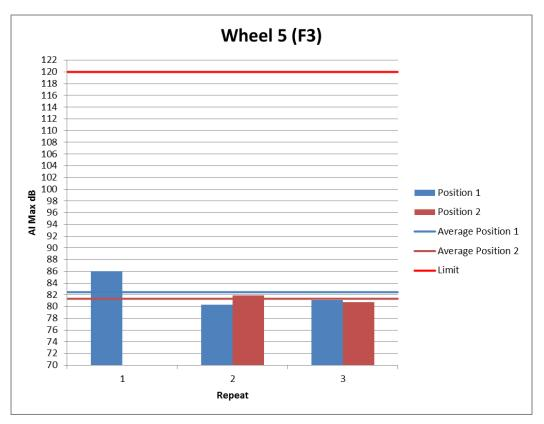
Figure 66: Individual Noise Levels for Wheel 5 (F3)
