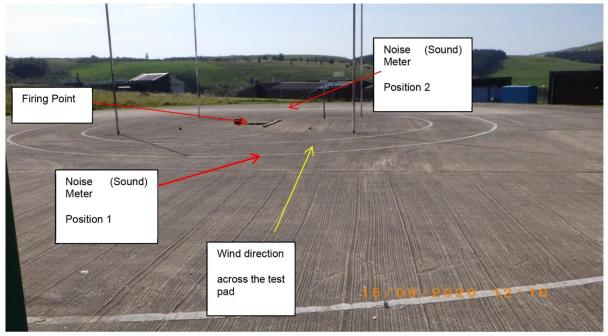
Photograph 2: Noise (Sound) Meter Positioning (at 8 m) for a Category 2 Firework
