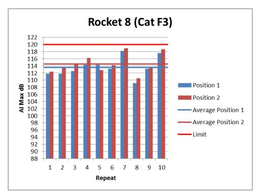
Figure 23: Individual Noise Levels for Rocket 8 (F3)
