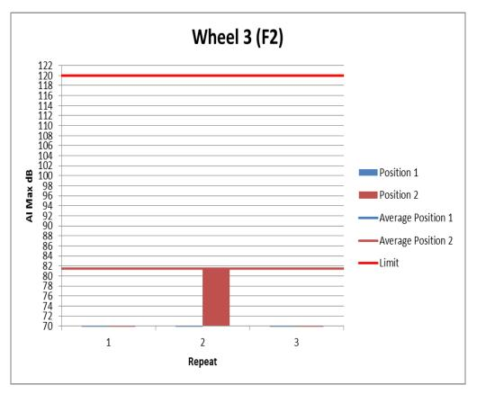
Figure 64: Individual Noise Levels for Wheel 3 (F2)
