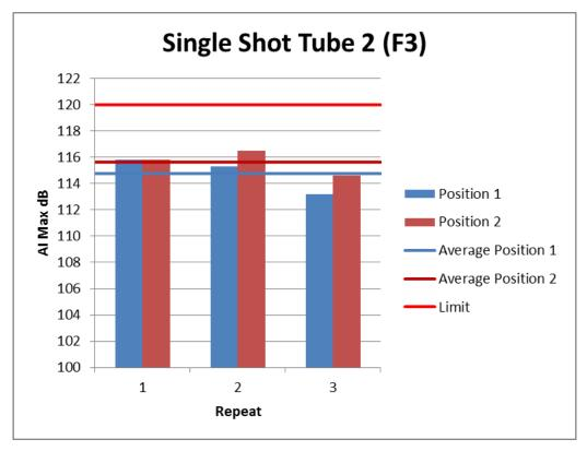
Figure 81: Individual Noise Levels for Single Shot Tube 2 (F3)
