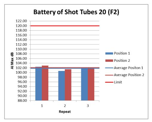
Figure 47: Individual Noise Levels for Battery of Shot Tubes 20 (F2)
