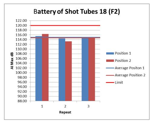
Figure 45: Individual Noise Levels for Battery of Shot Tubes 18 (F2)
