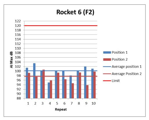
Figure 21: Individual Noise Levels for Rocket 6 (F2)
