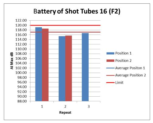
Figure 43: Individual Noise Levels for Battery of Shot Tubes 16 (F2)
