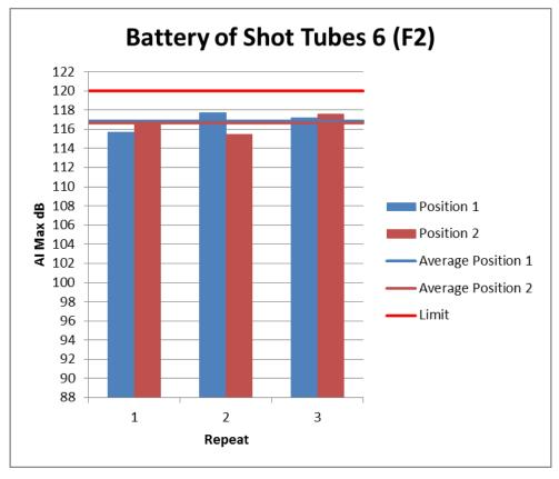
Figure 33: Individual Noise Levels for Battery of Shot Tubes 6 (F2)
