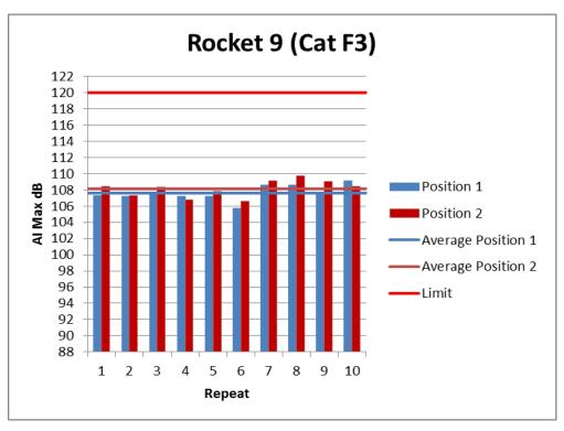
Figure 24: Individual Noise Levels for Rocket 9 (F3)
