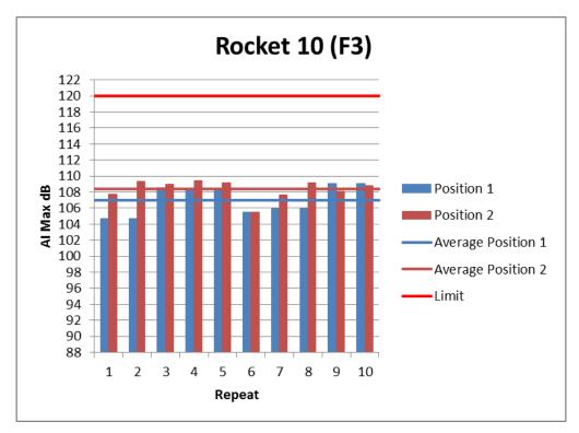
Figure 25: Individual Noise Levels for Rocket 10 (F3)
