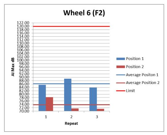
Figure 67: Individual Noise Levels for Wheel 6 (F2)
