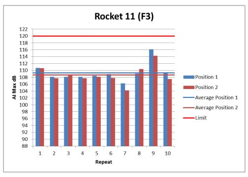
Figure 26: Individual Noise Levels for Rocket 11 (F3)
