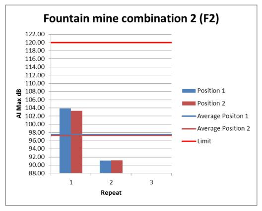
Figure 85: Individual Noise Levels for Fountain/Mine Combination 2 (F2)
