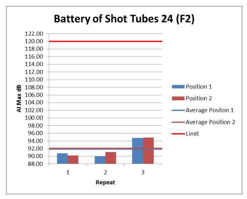
Figure 51: Individual Noise Levels for Battery of Shot Tubes 24 (F2)
