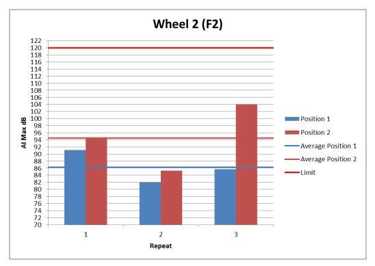
Figure 63: Individual Noise Levels for Wheel 2 (F2)
