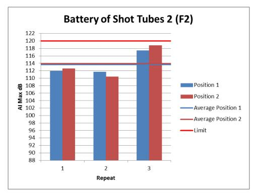
Figure 29: Individual Noise Levels for Battery of Shot Tubes 2 (F2)
