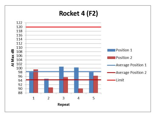
Figure 19: Individual Noise Levels for Rocket 4 (F2)
