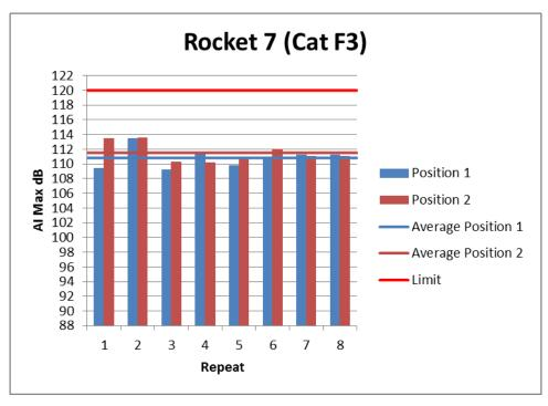
Figure 22: Individual Noise Levels for Rocket 7 (F3)
