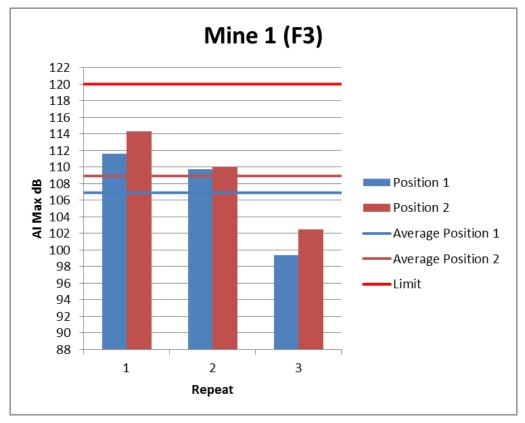
Figure 82: Individual Noise Levels for Mine 1 (F3)
