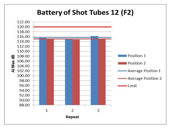
Figure 39: Individual Noise Levels for Battery of Shot Tubes 12 (F2)
