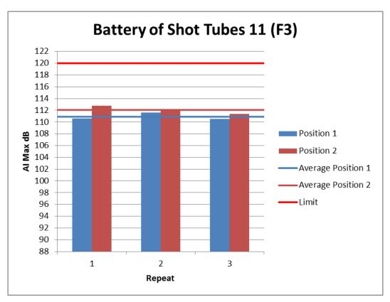
Figure 38: Individual Noise Levels for Battery of Shot Tubes 11 (F3)
