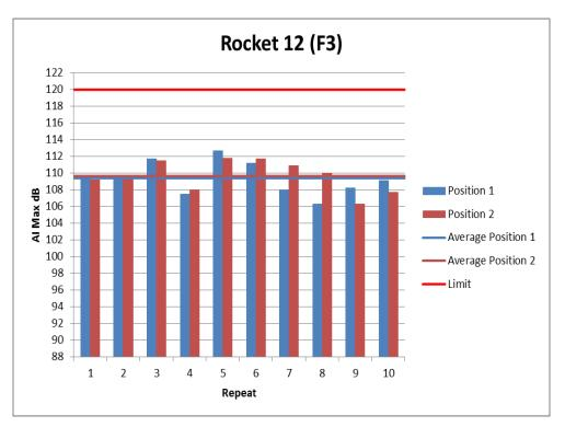
Figure 27: Individual Noise Levels for Rocket 12 (F3)
