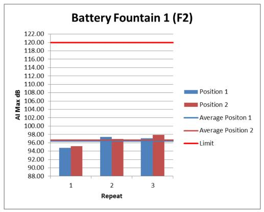
Figure 86: Individual Noise Levels for Battery of Fountains 1 (F2)
