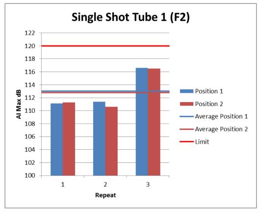
Figure 80: Individual Noise Levels for Single Shot Tube 1 (F2)
