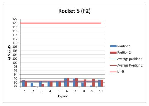
Figure 20: Individual Noise Levels for Rocket 5 (F2)
