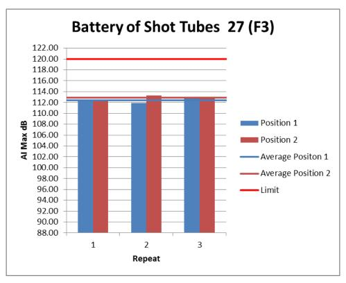
Figure 54: Individual Noise Levels for Battery of Shot Tubes 27 (F3)
