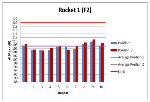
Figure 16: Individual Noise Levels for Rocket 1 (F2)
