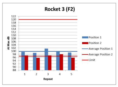
Figure 18: Individual Noise Levels for Rocket 3 (F2)
