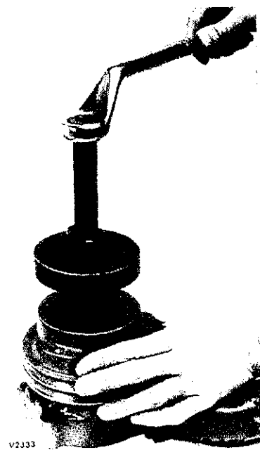
Fig 102 - Removing water pump pulley
