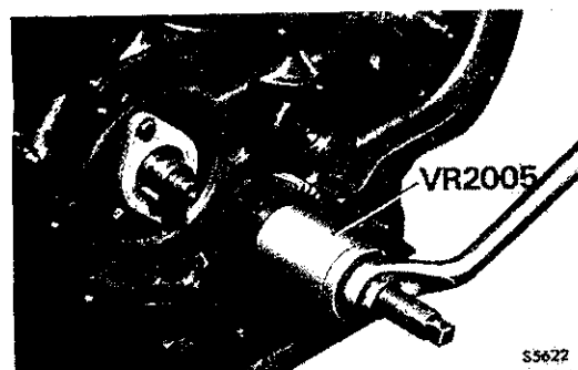
Fig 31 Installing crankshaft gear
