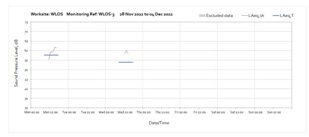
Note: Missing data throughout the week was due to loss of power supply to the monitor.
