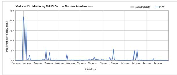
Note: High vibration levels measured at 09:00 on Monday 14<sup>th</sup> November was due to topsoiling and hydroseeding works undertaken in vicinity of the monitor.
