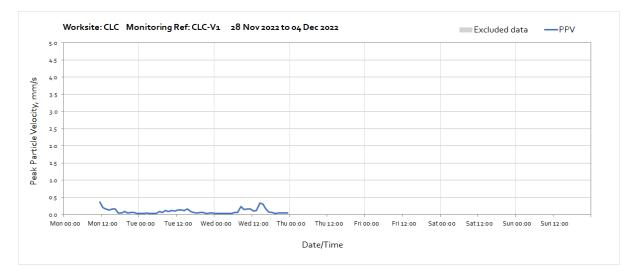
Note: Missing data from 00:00 to 11:00 on Monday 28<sup>th</sup> November till the end of the week was due to loss of data connection to the monitor.
