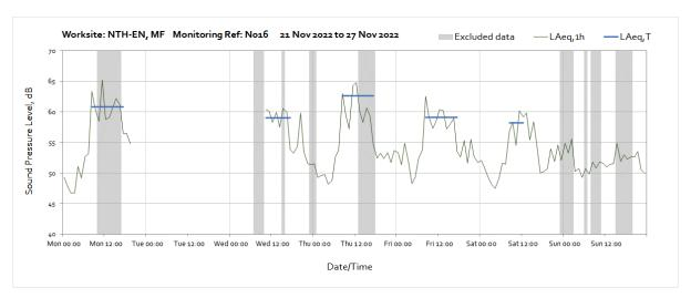
Note: Missing data between 20:00 on Monday 21<sup>st</sup> November and 10:00 on Wednesday 23<sup>rd</sup> November was due to a battery power failure which was resolved upon access being granted to the monitoring location.
