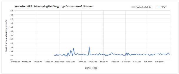
Note: Missing data from the beginning of the month until 18:00 on Tuesday 1<sup>st</sup> November was due to a loss of power caused by a depleted battery which were subsequently replaced.
