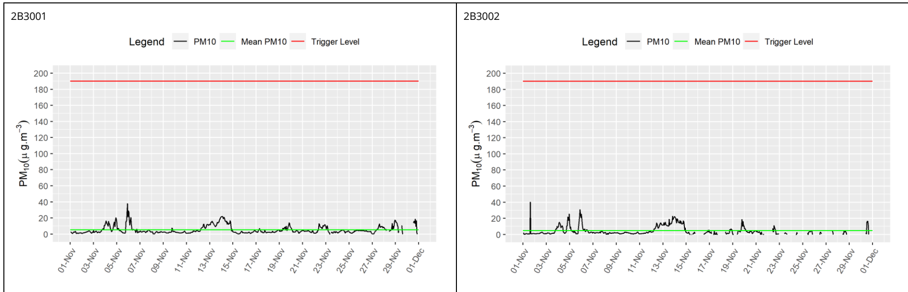
Figure 3: Construction dust 1-hour mean indicative PM 10 concentration for all dust monitors
