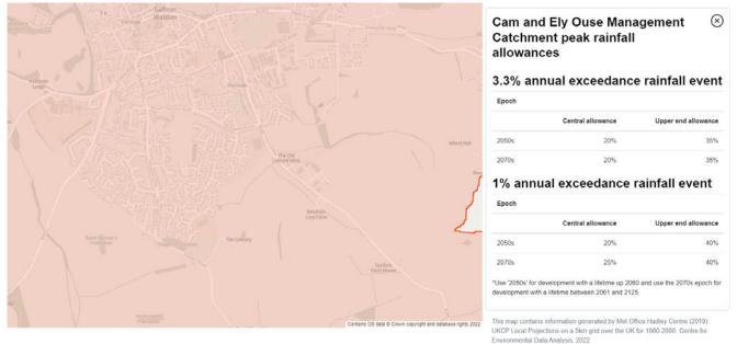
The full 40% climate change allowance has been included in the proposed storage design and this should be retained through the detailed design.
