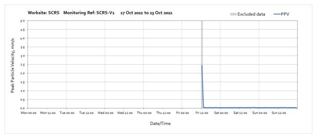
Note: Missing data between 00:00 on Saturday 1st October and 12:00 on Friday 21st October was due to damage of the fuse caused by vegetation clearance resulting in loss of power to the equipment.
