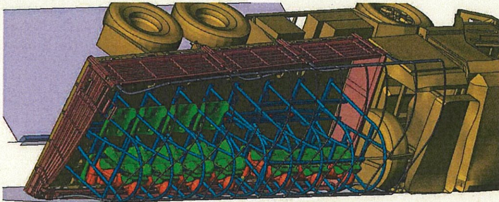
The rear roll hoops distort around the load bed frame
