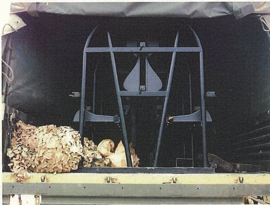
Figure 1 – Troop Carrying Vehicle Enhanced Seating (TCV ES) system, Mk 2, Ser No – ESK02243
