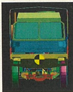
Fig. 2.6 : HX58 CAE model Centre of Gravity plots
