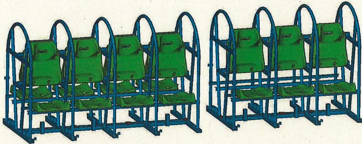
Fig 2.2 : TCVES Mk2 Seating Frame CAE model
