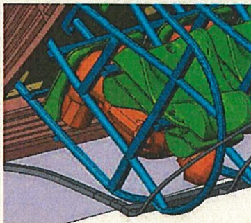
The rear roll hoops distort around the load bed frame
