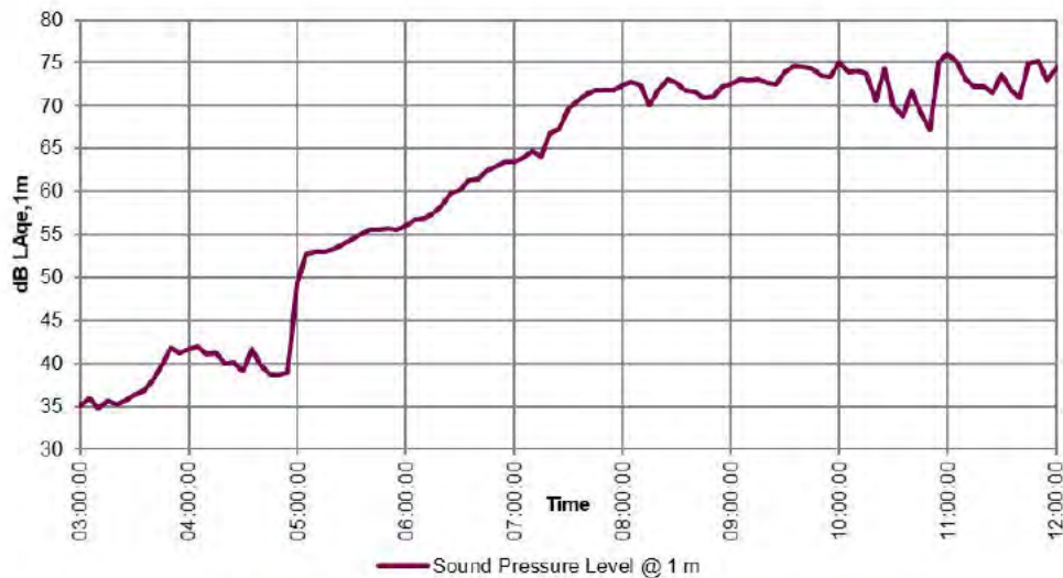
Figure 4.1: PV Inverter Noise Emissions Over Time
