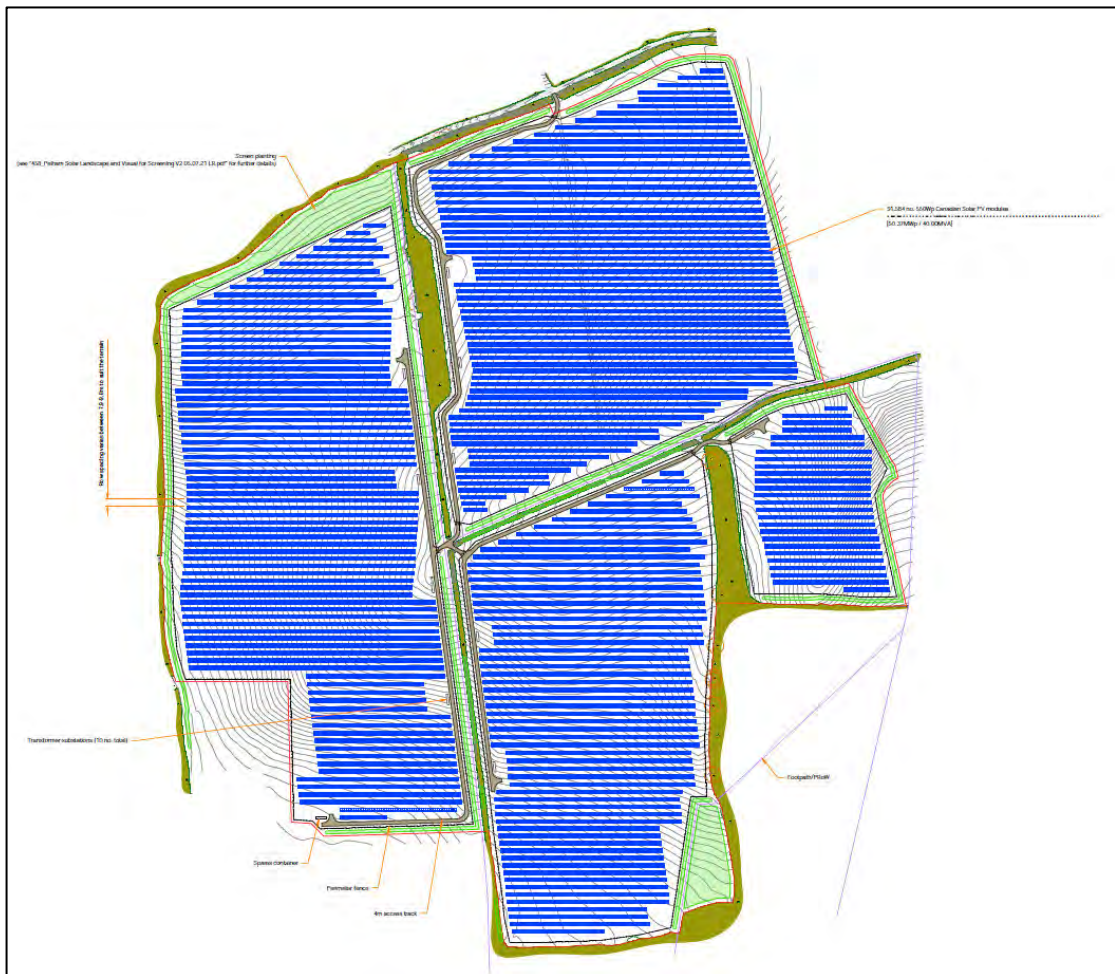
Figure 1 Proposed PV layout
