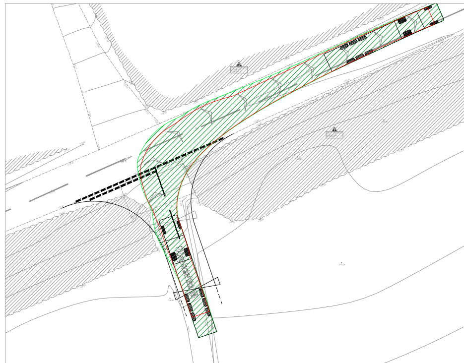
16.5m ARTICULATED VEHICLE RIGHT TURN OUT MANOEUVRE
