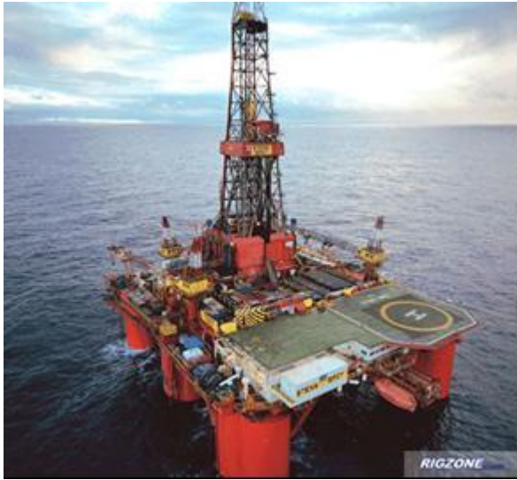
Figure 2.2 – Typical semi-submersible rig 5
