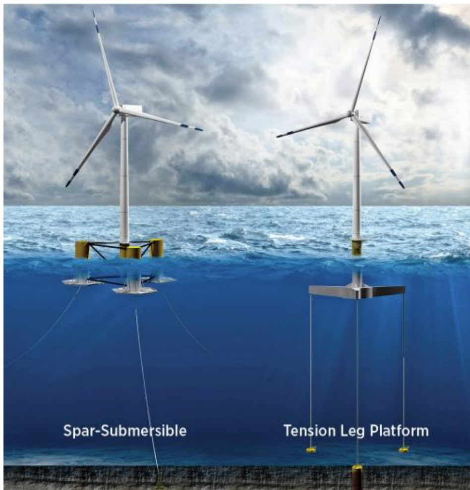
Figure 3.14: Examples of potential substructures for the Avalon floating OWT (image from IRENA)
