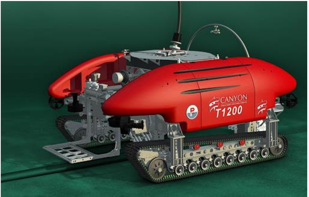
Figure 3.5: Canyon T1200 jetting trencher
