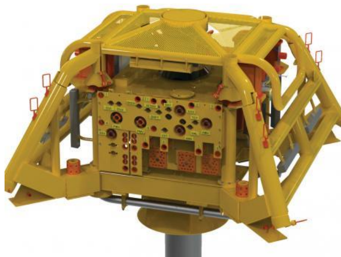
Figure 3.3: Example of Xmas Tree Within Protection Structure
