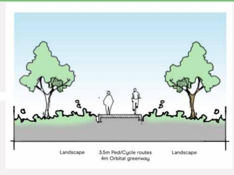
Pedestrian & Cycle Routes - Street Section Sections are illustrative and do not indicate differing ground levels.
