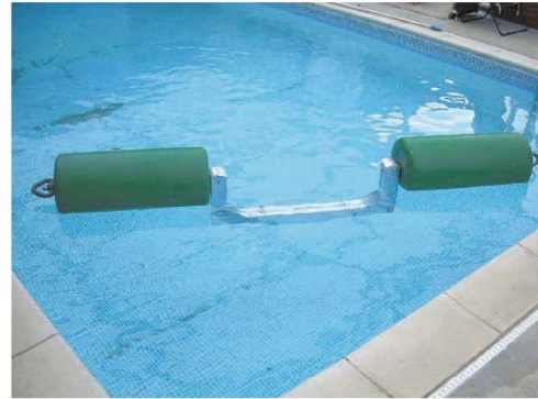
b A canoe stirrup inserted into a barrel chain can allow canoeists to negotiate through a boom to shoot a weir, seen here in a swimming pool.
