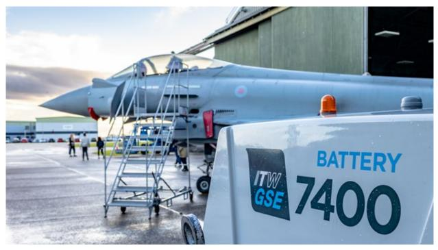
Forty new ground power units (GPUs), using the same battery packs found in Nissan Leaf electric cars, will soon power Typhoon aircraft on the ground at RAF Coningsby and RAF Lossiemouth.
