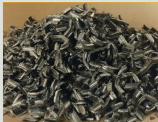
ILW Magnox fuel cladding swarf
