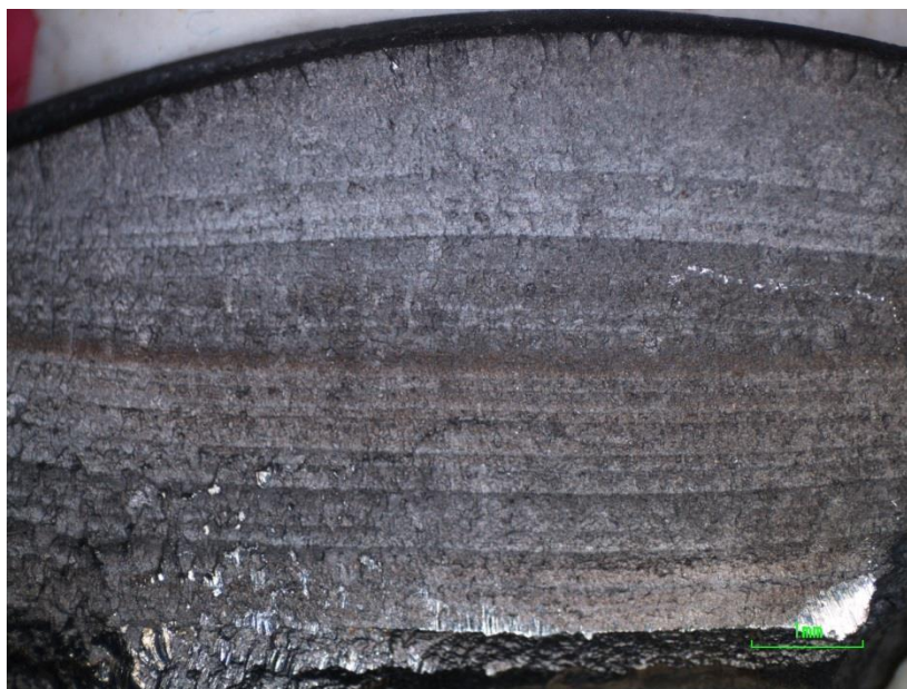
Figure B-6: Beach marks in a steel component.
