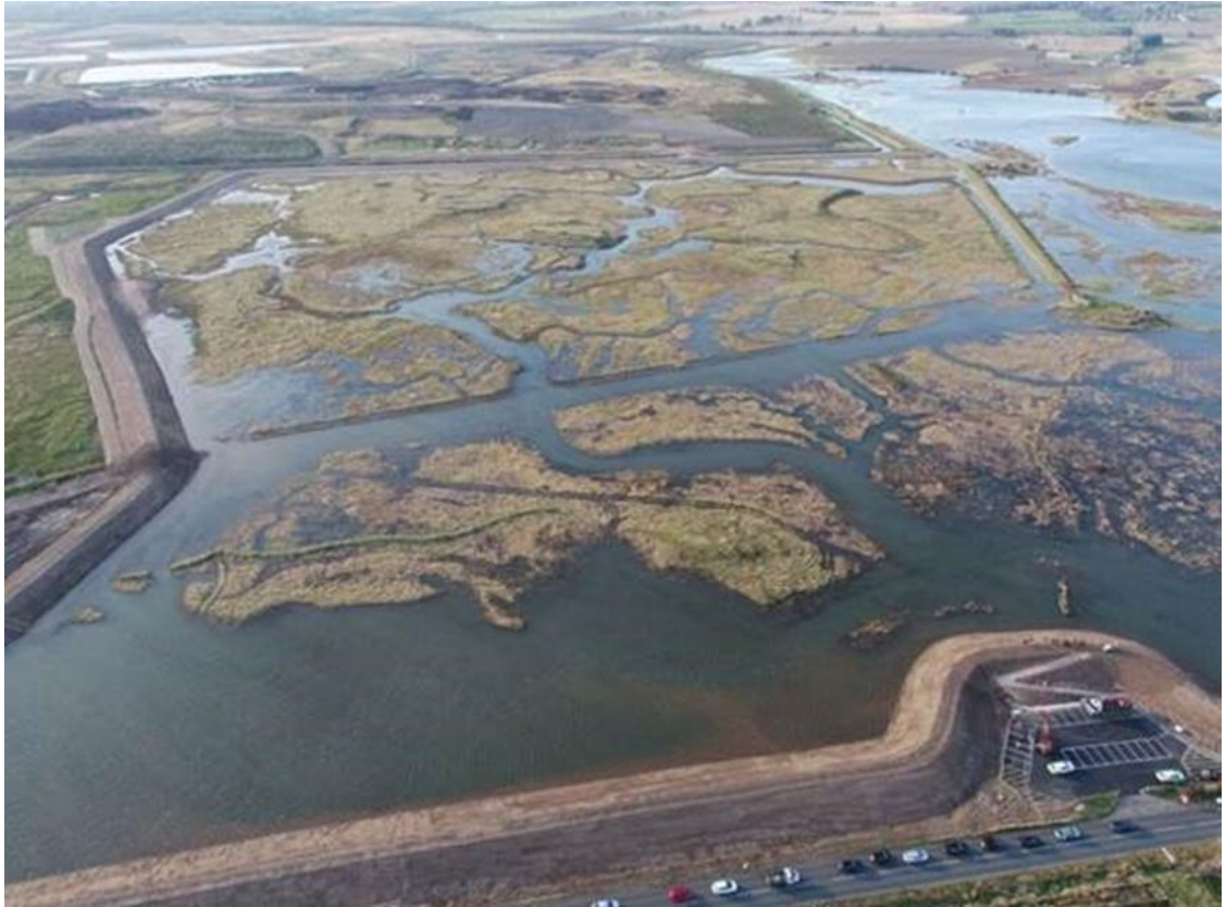
Figure 2: Greatham South Scheme. Creation of intertidal habitat, predominantly upper salt marsh with mudflats and tidal creeks after existing embankment was purposefully breached and realigned.
