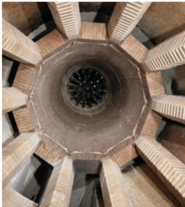
Figure 4: Lance array at the top of a PFR kiln (photo courtesy of Lhoist UK)
