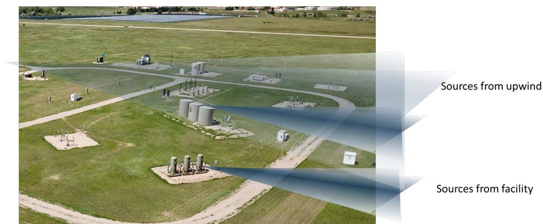
Figures 3.2 to 3.5 show different sensing approaches used in estimating facility emissions. These approaches involve either continuous monitors (permanently installed systems making regular measurements over an extended period of time) and/or survey methods (intensive measurements made during short campaigns on a single or periodic basis).
