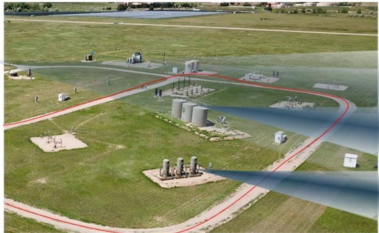
**Figure 3.5: Survey methods: Using a flux plane method to survey the emissions plume from a facility**
