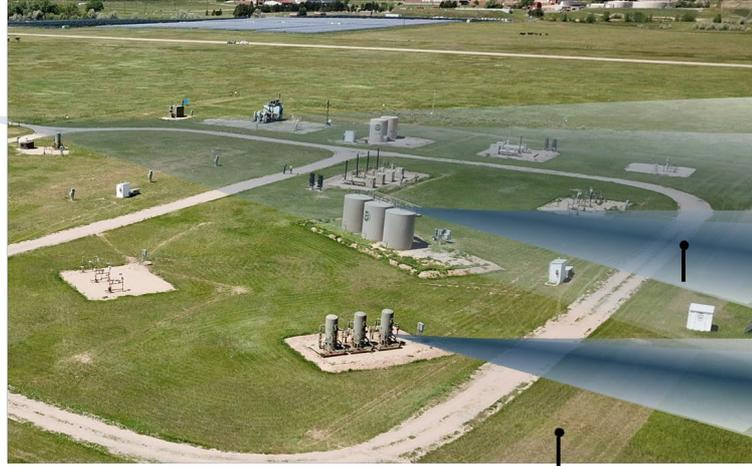
**Figure 3.3: Continuous monitors or survey methods: Using line (laser) sensors (yellow lines) to measure concentrations in or near the emissions plume from a facility**
