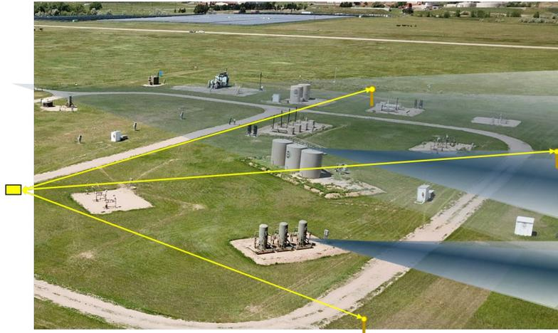
**Figure 3.4: Survey methods: Using a concentration survey of the emissions plume from a facility**
