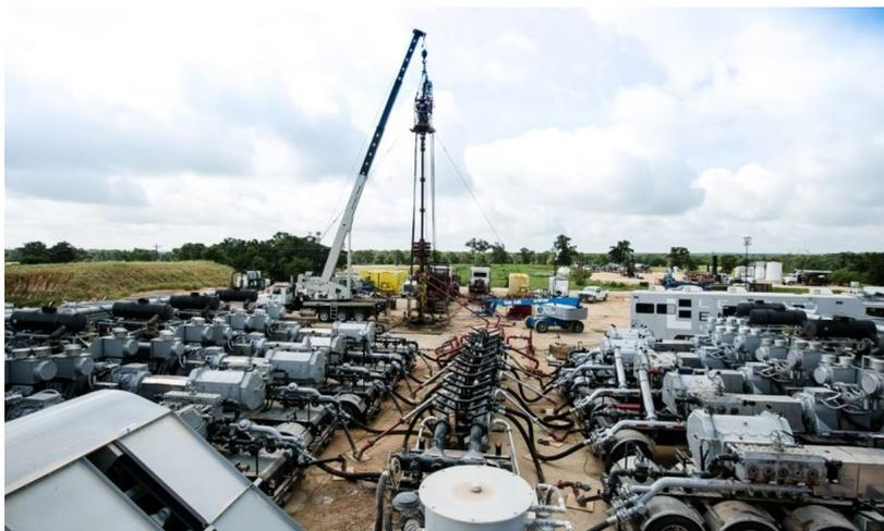
Figure 4: Fracturing equipment surface set-up (ICOTA, 2022)
