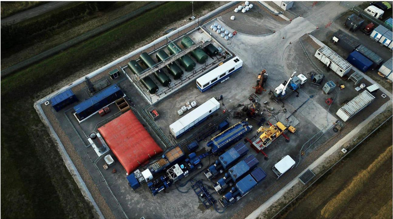
**Figure 12: Surface equipment set-up for low volume hydraulic fracturing (Lincolnite, 2021)**
