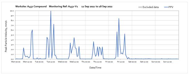
Note: High vibration levels measured throughout the week was due to excavation works occurring within 20m of the monitoring station.
