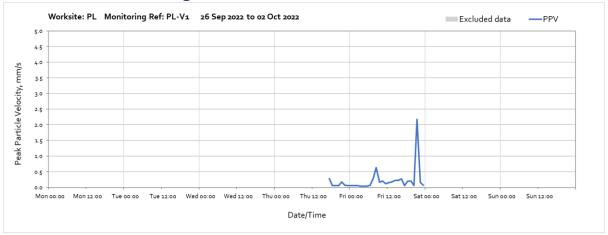
Note: Missing data from the beginning of the month till 29<sup>th</sup> September was due to monitor been removed from the site for relocation. The monitor was reinstalled on 29<sup>th</sup> September. High vibration levels measured due to relocation of the monitoring station.
