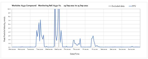
Note: High vibration levels measured throughout the week was due to excavation works occurring within 20m of the monitoring station.
