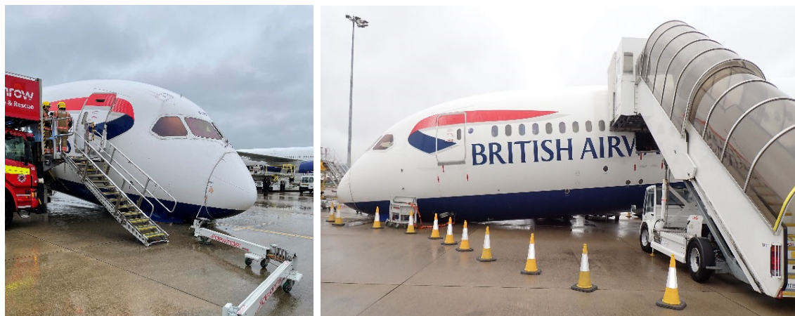
Figure 2 View of right and left side of the aircraft following NLG retraction
