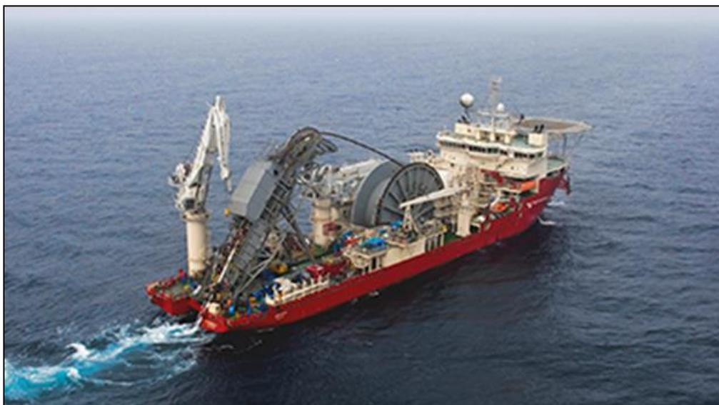
For some of the smaller diameter pipeline, flexible and umbilical sizes, recovery could also be achieved by using a CSV/ Dive Support Vessel (DSV) with a reel drive system on the deck. Depending on the size of the vessel deck, multiple reels can be used, as shown in Figure 5.
