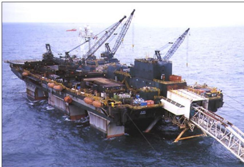
It should be noted that there is no industry track record of reverse S-lay of concrete coated pipe. There are also potential issues with the deterioration of the concrete coating over time which would hinder pick up of the pipe and may result in sections falling off during recovery.
