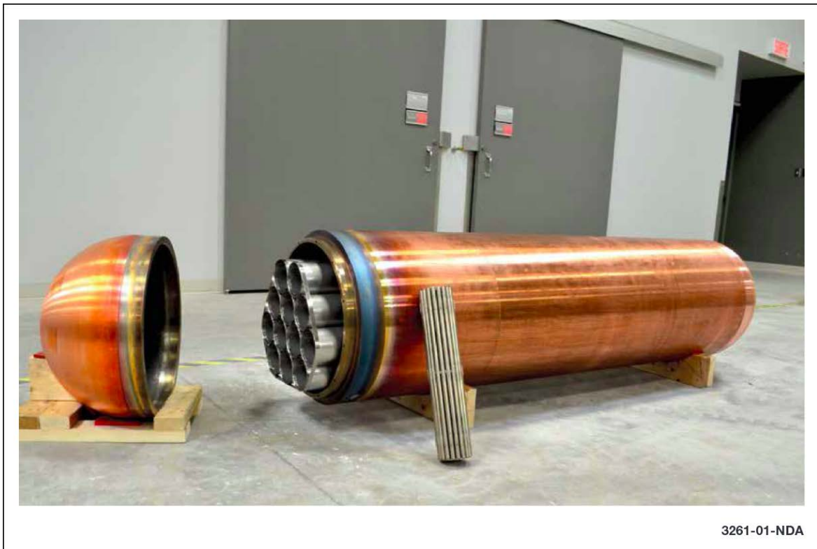
Figure A2-3: Full-scale test model of a NWMO copper-coated steel container [A2.3].
