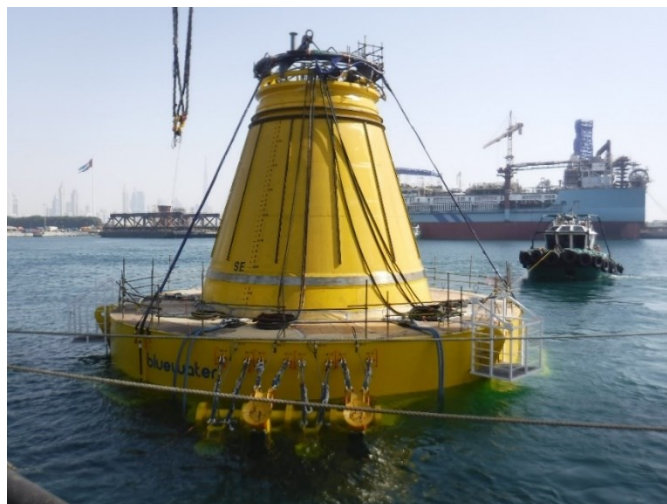
Figure 3:3 - Disconnectable Turret Buoy (DTB)
