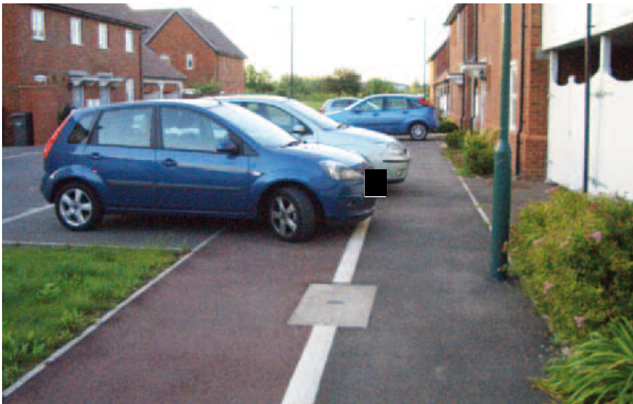
1.5m setback design allows vehicles to obstruct footway/cycleway
