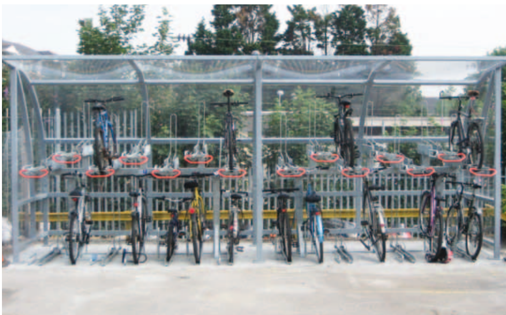
Two tier racks within covered cycle shelter
