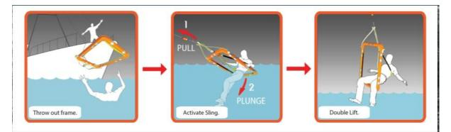
The Markusnet is a unique means to retrieve a man overboard manually, as well as, by crane, when every second counts, using the vessel deck as the rescue base.
