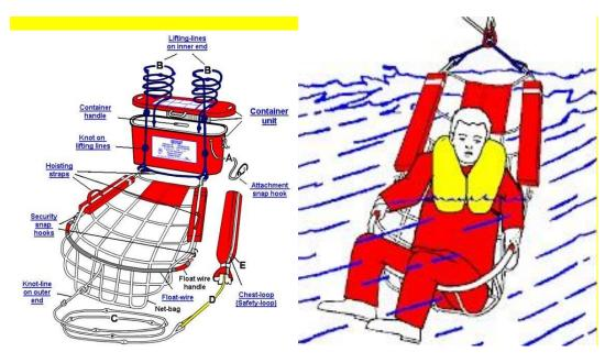
The Markusnet is a revolutionary rescue device that enables one person to react immediately and effectively to a man overboard situation anywhere along a ship's side or quay and two rescuers to lift the victim in seconds, despite the freeboard height of vessel, thereby greatly increasing the casualty's chances of rescue. It is also an ideal teaching tool to prevent man overboard hazards and tragedy, as well as, to train your crew to becoming professional inwater MOB rescue team.
