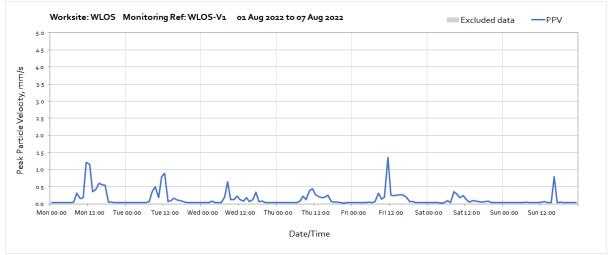
Note: High vibration levels measured throughout the week was due to Hydrophraise works occurring within 10-50m of the monitoring station.
