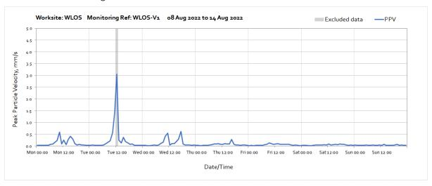
Note: High vibration levels measured between 11:00 and 12:00 on  $9^{th}$  August were due to Hydrophraise works occurring within 10-50m of the monitoring station.
