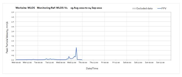
Note: High vibration levels measured at 17:00 on 31st August due to Hydrophraise works occurring within 10-50m of the monitoring station.
