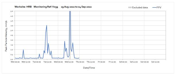
Note: High levels of vibration measured from 13:00 until 14:00 on Wednesday 31<sup>st</sup> August were due to pile mat preparation activities undertaken near to the monitoring station. The monitoring station is mounted on a kentledge block along the hoarding in an area of disturbed ground, vibration is likely to be amplified compared to what is experienced at building. Attended monitoring has been booked to acquire more representative data for the receptor.
