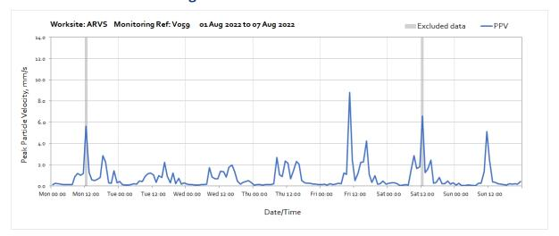
Note: High levels of vibration measured from 10:00 until 11:00 on Friday 5<sup>th</sup> August were due to utilities work being undertaken in close proximity to the monitor. Vibration levels at the nearest receptor will be lower.
