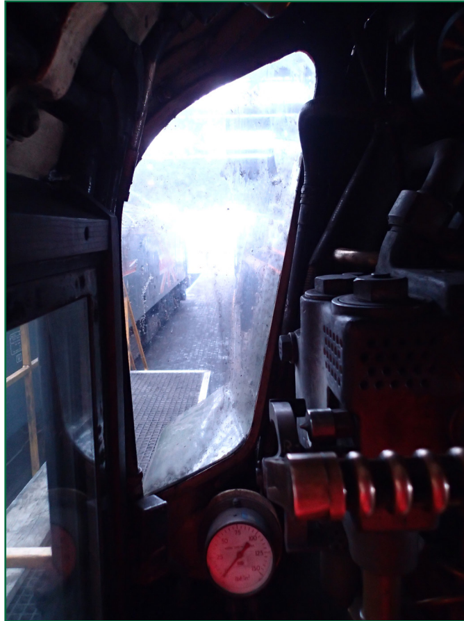
Figure 13: The driver's windscreen on Tangmere. Note that this photograph was taken with the train at a stand within a depot and does not show the driver's forward visibility on 7 March 2015
