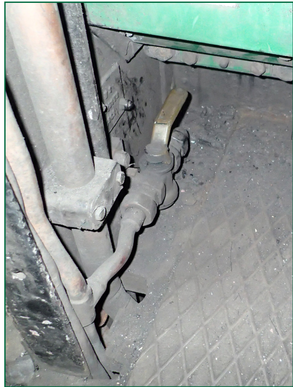
Figure 12: The AWS isolating cock shown in the closed position
