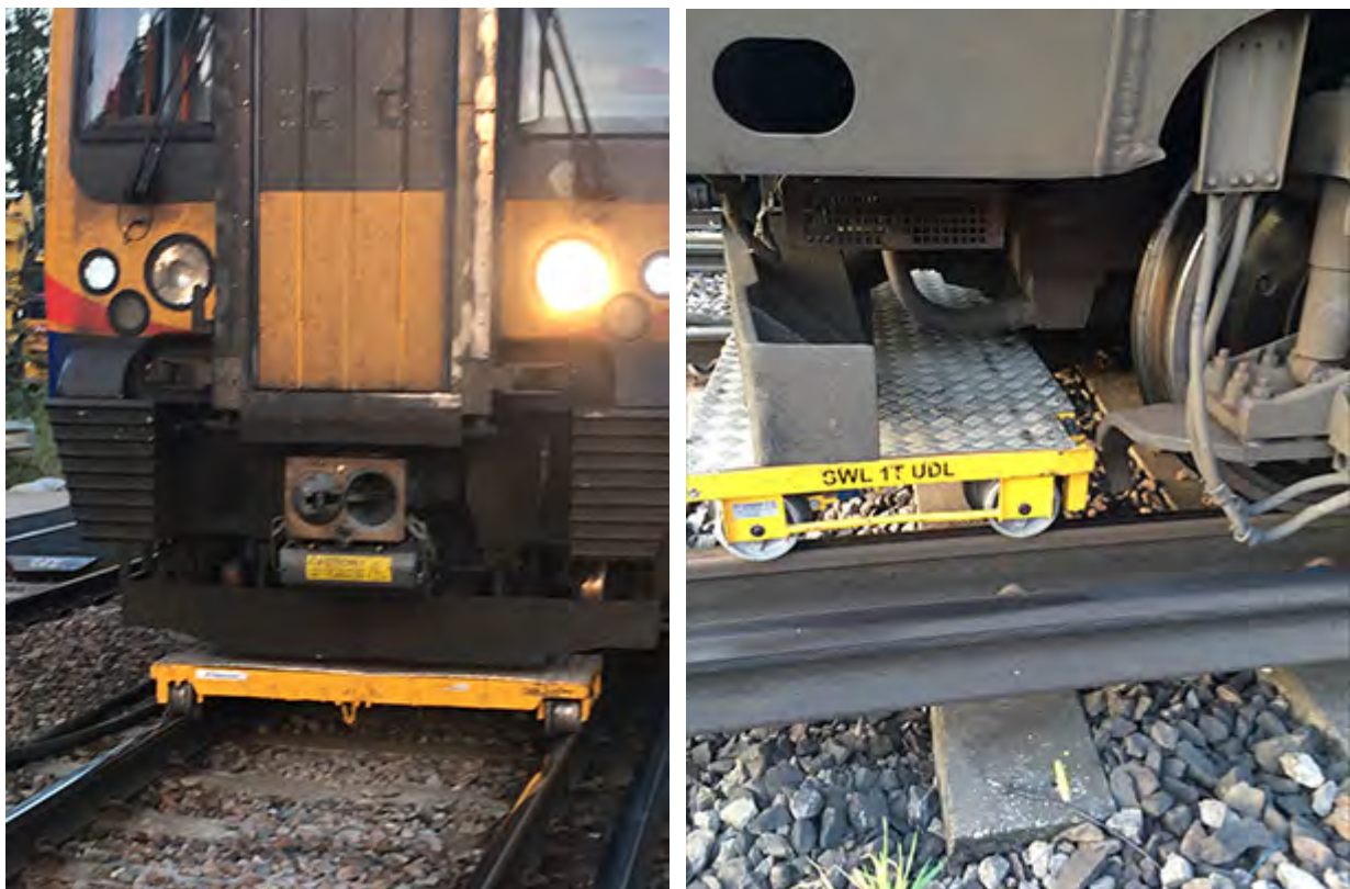
Figure 18: The train and hand trolley after the collision at Twickenham (courtesy of Network Rail)
