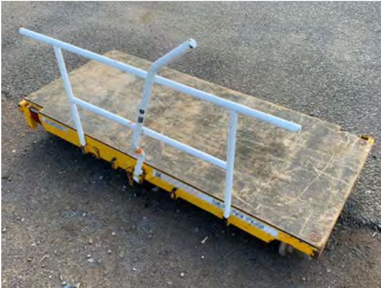
Figure 6: The type of hand trolley struck by train 1C00 (courtesy of Network Rail)
