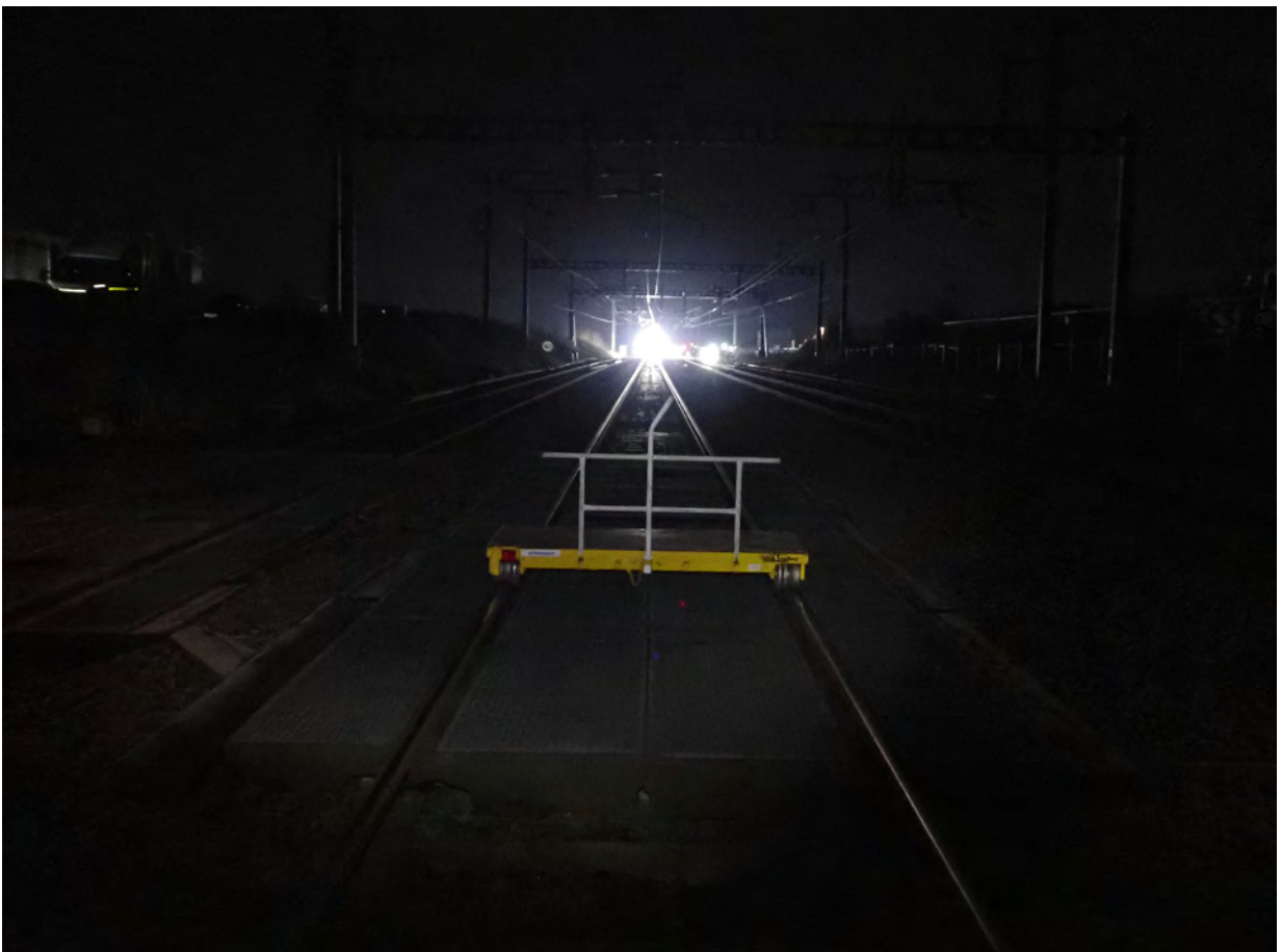
Figure 13: A hand trolley, with no illuminated red lights, on the road-rail access point in darkness during the reconstruction (top image) and illuminated by torch light for comparison (bottom image)
