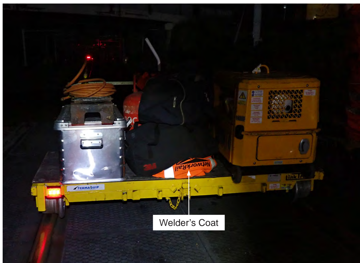
Figure 11: A reconstruction of how the hand trolley was loaded by the COSS and the welder after completing the repair
