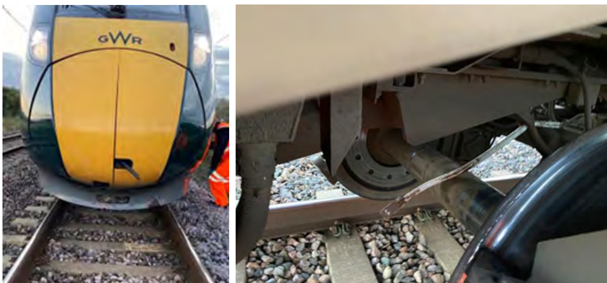
Figure 2: The train once stopped and the handle from the hand trolley wedged under it (courtesy of Network Rail)
