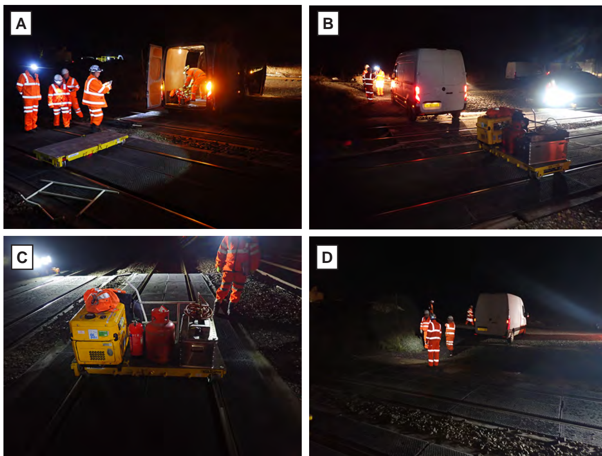
Figure 7: A reconstruction undertaken following the accident, showing the van reversing onto the road-rail access point to load equipment onto the hand trolley and then parked afterwards
