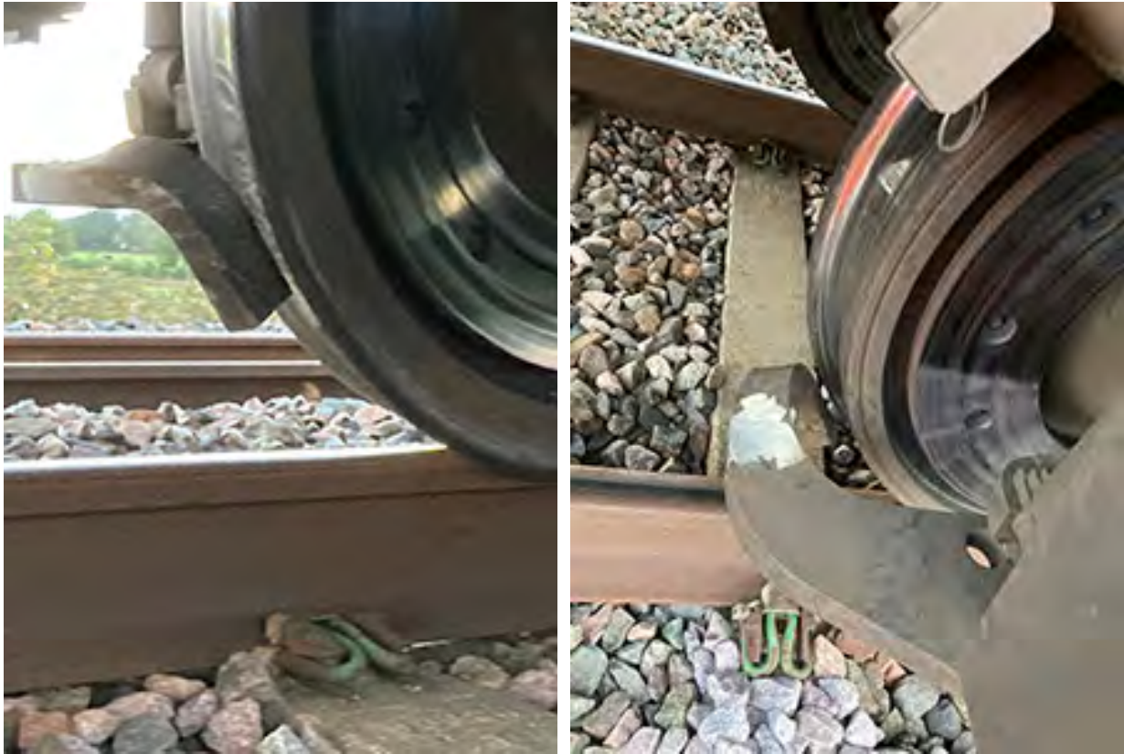
Figure 16: The damaged lifeguards on the leading vehicle (courtesy of Hitachi Rail)
