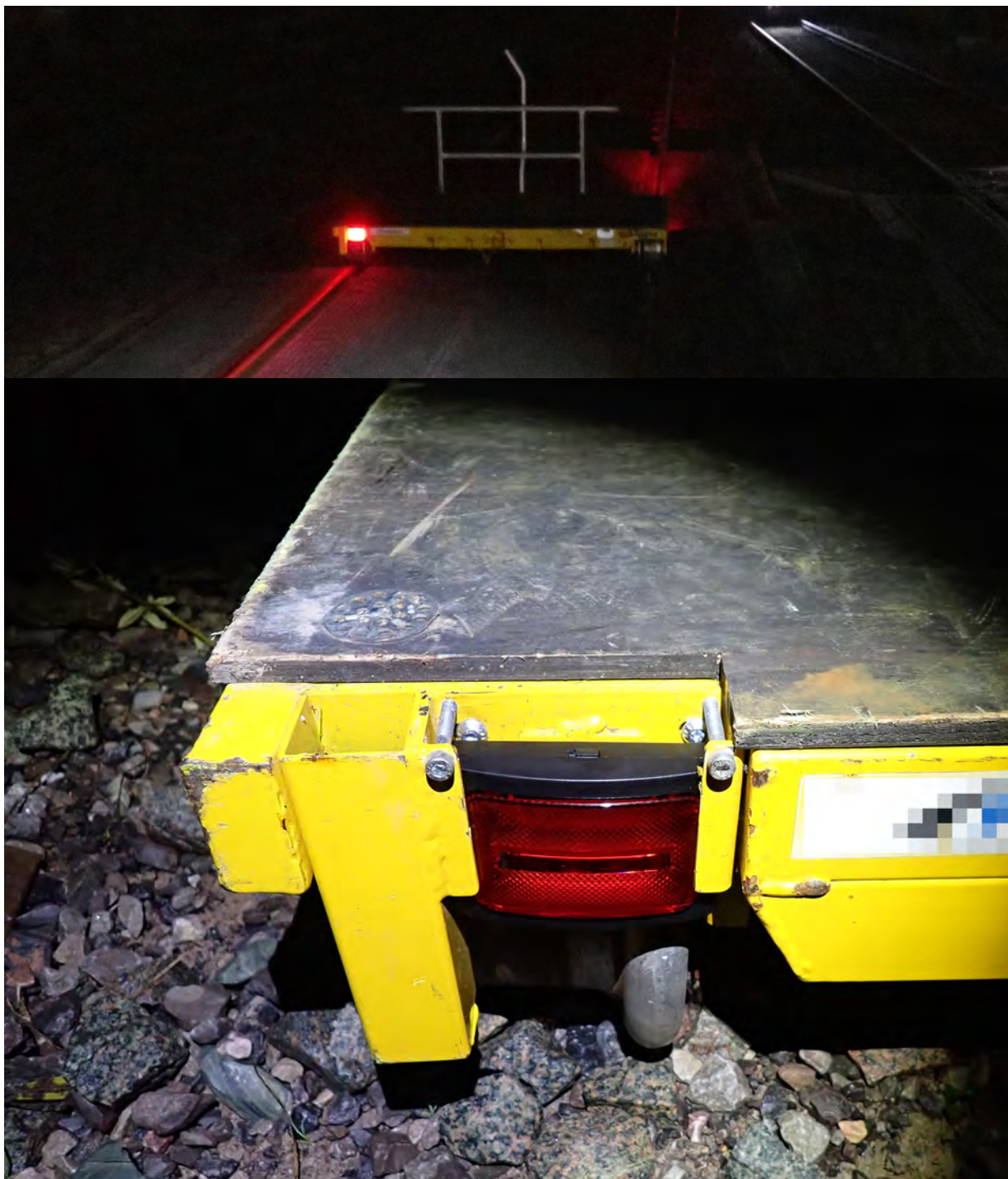
Figure 14: The red-light units on the same model of hand trolley.
