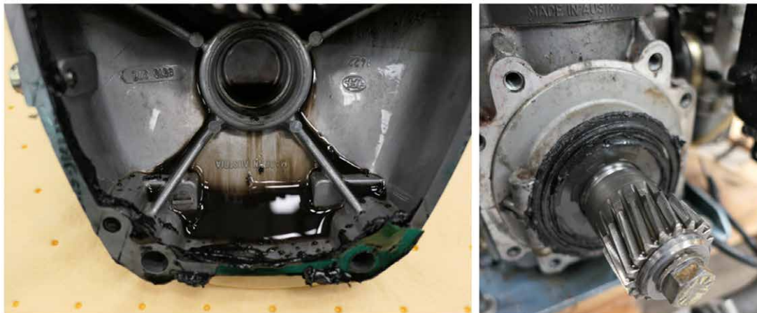
Figure 3 Left – exuded sealant inside casing Right – sealant on crankcase interface
