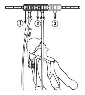
**1. Full-Body Safety Harness** Use a full-body safety harness attached to the access traveller with lock. Fullbody safety harness must meet UKCA mark/CE mark till 31 December 2022 or an alternative standard which provides equivalent levels of safety, suitability and fitness for purpose when in use
