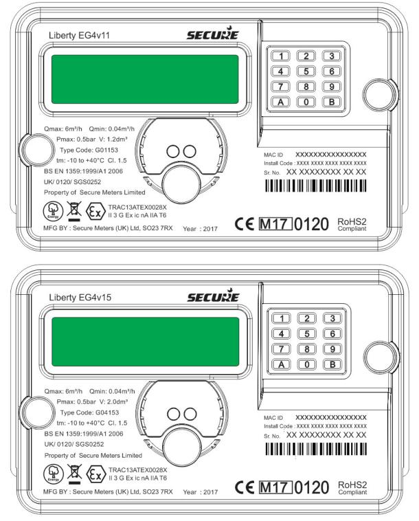
Drawings showing Gas meter markings, please note a 2D barcode may be used in place of the 1D barcode shown.
