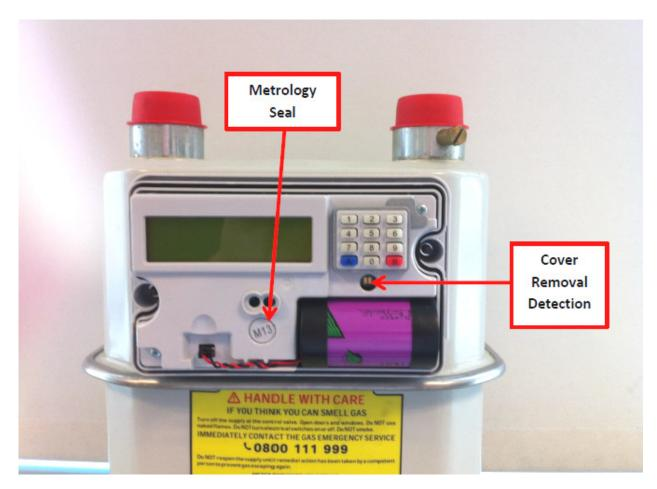
Removing the front cover allows access to battery the inner cover's Metrology seal prevents its removal without destroying the seal.
