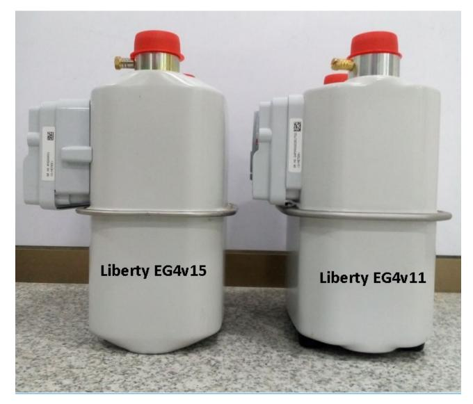
The differences between the two variants are most evident when viewed from the side. The 2dm<sup>3</sup> EG4v15 G04153-Z01, approved in this issue of the certificate, has a deeper electronic index to accommodate an integration plate and idler gear. The 1.2dm<sup>3</sup> EG4v11 G01153-Z01 meter, approved on the initial certificate, is fitted with black plastic feet.
