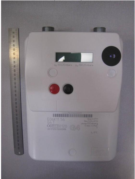
Meter incorporating fixed pressure correction (identified by  $p_b$  and  $p_a$  markings on the module). The photograph shows a meter with tb=0<sup>o</sup>C the base temperature is marked on the front of the base meter .
