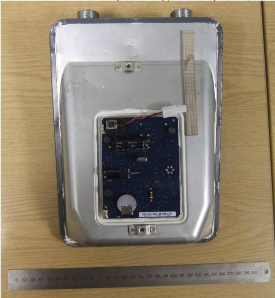
Meter with valve close on battery removal facility (characterised by button cell)
