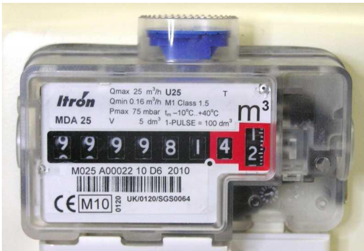
Pulse Ready Meter Index showing blue security seal location. The Index is shown without the optional 45-0000 pulse module fitted.
