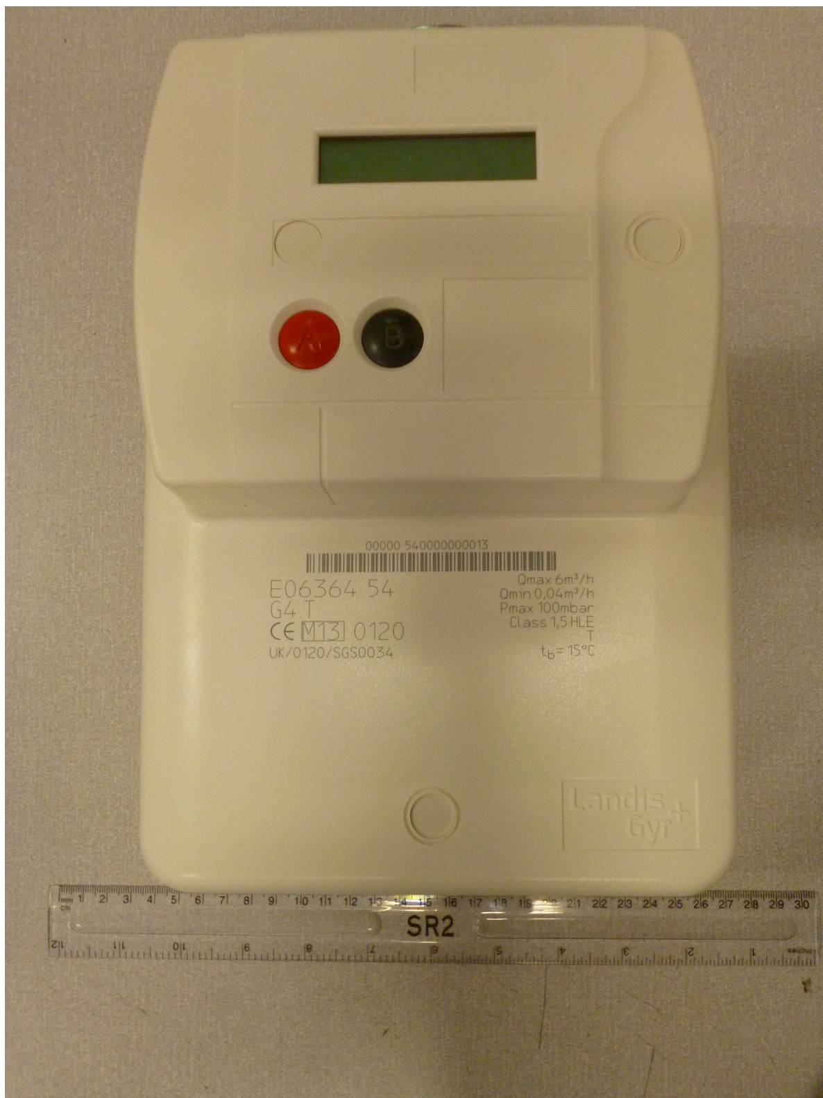
Meter E06364 54 with temperature compensation
