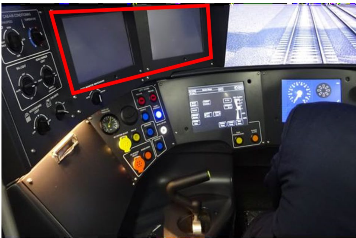
Interior of the class 710 driving cab with the DOO monitor screens highlighted (image courtesy of Arriva Rail London).
