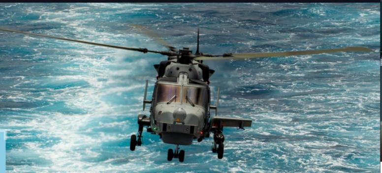
Successful Ship Helicopter Operating Limitations (SHOL) trials have proven that the Wildcat HMA Mk 2 can operate fully loaded with its newest missile systems in a range of challenging conditions at sea.
