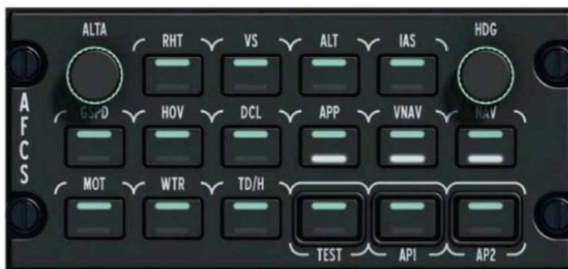
Figure 1 Autopilot Control Panel
