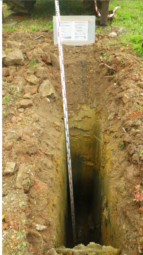
TP2A06 Trial Pit. Depth 3.3m
