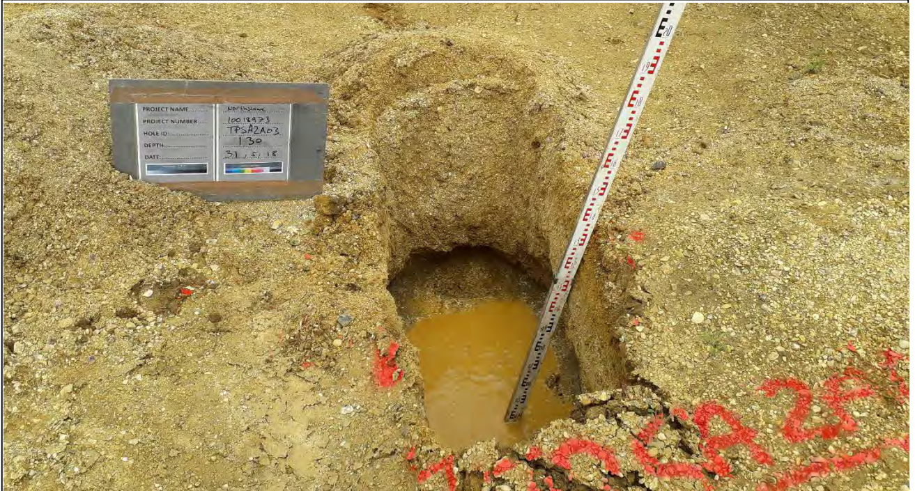
TPSA2A03 Trial Pit. Depth 1.30m
