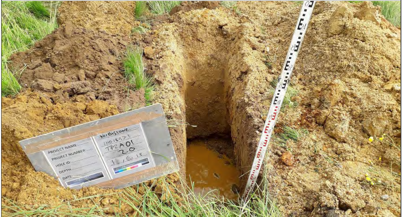
TP2A01 Trial Pit. Depth 2.0m
