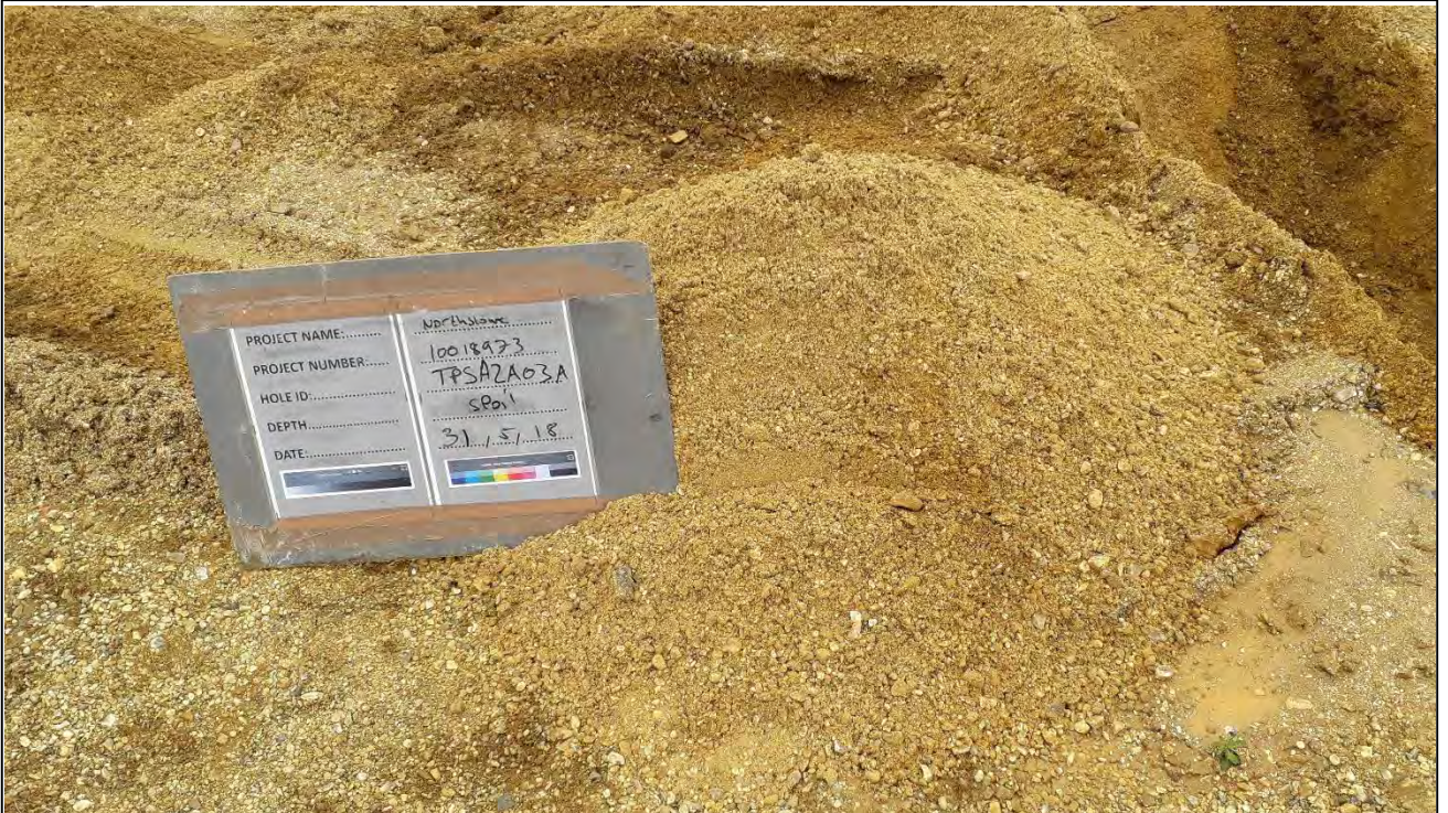
TPSA2A03A Trial Pit Spoil
